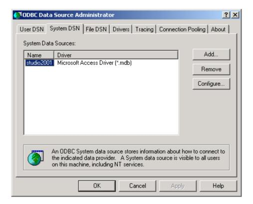
This screen shot shows a typical default install of the sample iNETstore database. If you have installed iNETstore multiple times, there might be additional data sources. If you are unsure which database to use, click on the 'Configure' to see current settings. To add a new data source, click on 'Add'.
